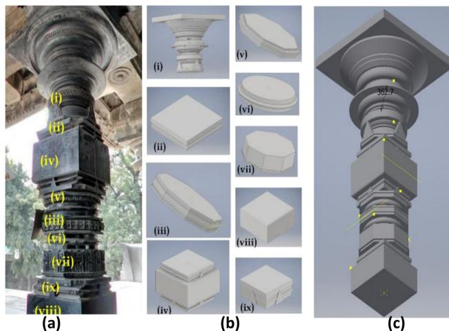
Fig.2. (a) Column with numerical Geometrical segregation (b) Individual component modelling (c) Concatenation of all the individual components
