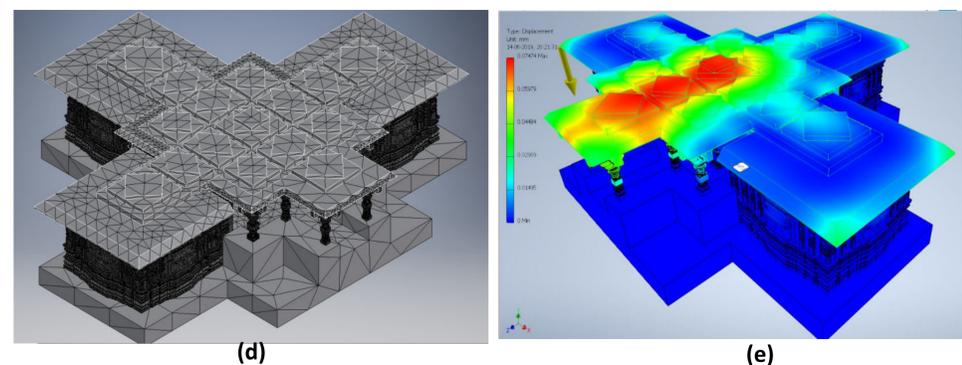
Fig.5. Column type-1 (a) meshing, (b) Von-misses stress and (c) displacement due to its self-weight. Complete temple (d) meshing, (e) Displacement due to gravity
