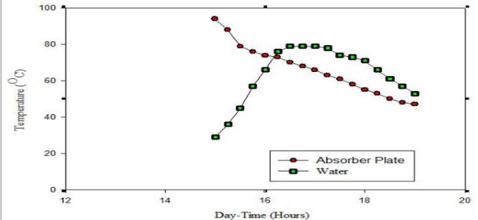
Figure 3. Variation of absorber plate and water temperature with time during heat retention test
